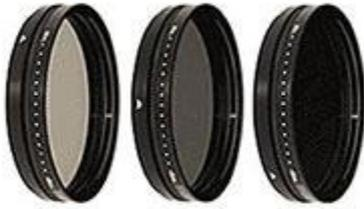
A neutral density filter is darkened over its entire surface to reduce the amount of light getting to the sensor, thus decreasing the shutter speed and increasing exposure time. They can be obtained in different strengths to achieve different creative ends, usually to create effects such as blurring or smoothing moving water or clouds. Or they can be used to “remove” people from a scene as, over the time of a lengthy exposure, moving people will not show up on the final image.
